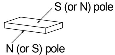
To check the polarity alignment a test magnet must be passed over the series of magnets. All magnets in the series must attract the test magnet or all must repel the test magnet. In case of any inconsistency the offending magnet(s) must be corrected or the DBR4-MCT will not work function correctly.
