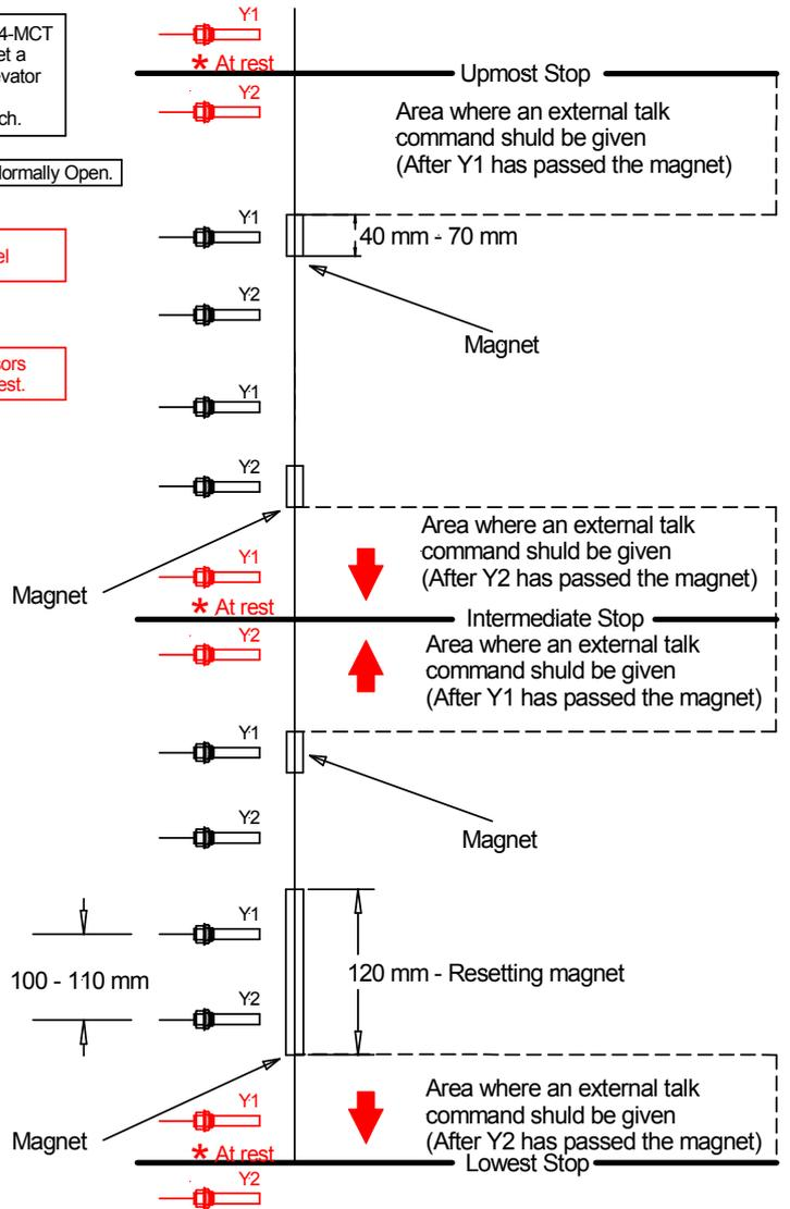
Attention: If the 120 mm magnet (at the bottom stage) consists of a series of smaller magnets laid consecutively then it is essential to ensure that the polarities of the magnets are aligned correctly, as follows:
